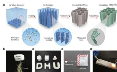
Figure 1. (a) Schematic illustration of the fabrication of FIBER NFAs. (b) A  $20\text{-cm}^3$  FIBER NFA ( $\rho = 0.12 \text{ mg cm}^{-3}$ ) stands on the tip of feathers. (c) FIBER NFAs with diverse shapes. (d) The water retention capacity of the nanofibrous hydrogels (NFH). A sample of squashed and dried NFH of  $\sim 10 \text{ mg}$  could hold  $\sim 5 \text{ g}$  of water. (e) Ceramic nanofibrous aerogels heated by a butane blowtorch without any damage.
